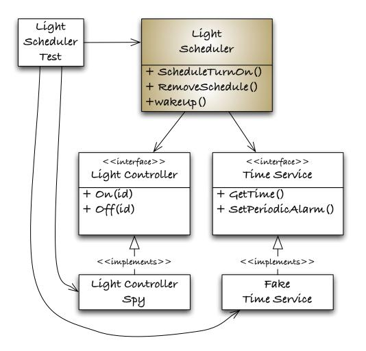
The test case takes the place of the client of the LightScheduler. The FakeTimeService replaces the TimeService during test as the LightControllerSpy does for the LightController. The LightScheduler has no idea that it is not working with test versions of its collaborators.
