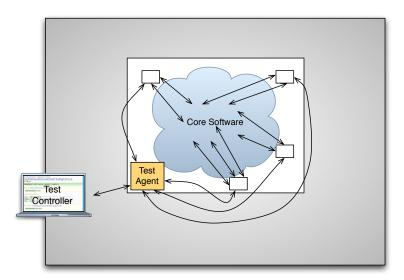
The test agent can generate events and capture responses at appropriate test points near the edges of the system and between subsystems. A test controller tells the test agent the events to simulate and the system states and responses to collect. Let's see how to use FitNesse to create a Test Controller and Test Agent.
