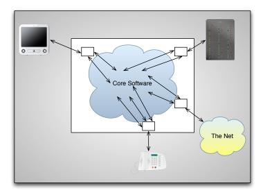
With the core application talking to the hardware and OS through interfaces, test implementations can be substituted for a test build. This diagram illustrates how a product is configured during test. Production drivers are substituted with drivers that can simulate input and capture outputs.
